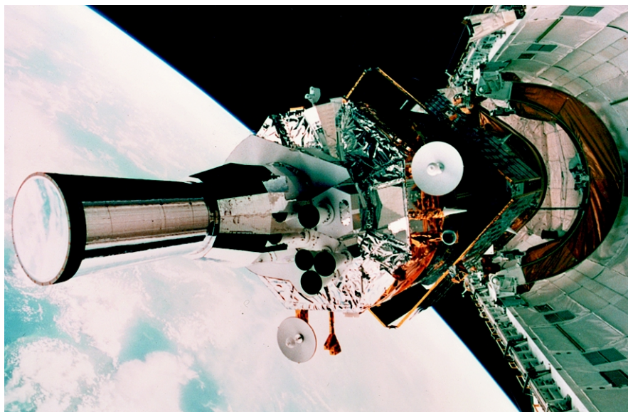
Defense Support Program satellites, such as this one launched in November 1991 from a space shuttle, provide early warning of missile launches.
